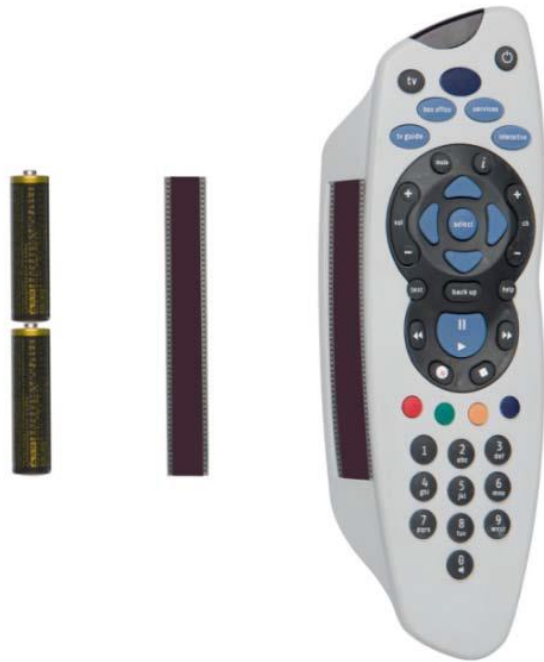
DSSC-powered remote control
